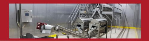
After feet got cut, they arrive to feet processing department. Firstly they go through temperature controlled scalders to make feet skin softer for an easier deskinning operation. Feet deskinners follows this procedure. According to capacity it is possible to automatically divide the feet to go through more than one machine. If desired, quality control could be done on a belt conveyor. Finally feet without skin got chilled with a screw conveyor inside cold water.
