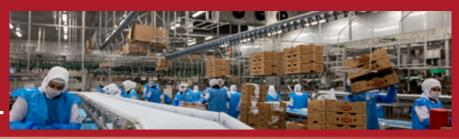
Chilled birds got packed as whole birds or portions according to their quality and weight. Kromeka sorting lines gives good results even in the high capacity lines with transfer machine from air chiller to sorting line, highly accurate weighing system and quality grading system with camera control.
