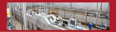
Defeathering department houses equipment that executes first processing on birds. The main operations are stunning, killing, bleeding, head removal, scalding, plucking and hock cutting. These primary operations on the birds have very important effects on quality of products.
