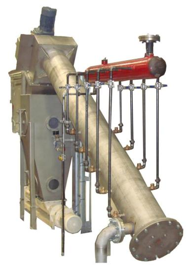
**Function:** To coagulate continuously the raw blood flow with injected direct steam into a blood clot which is ready for further processing/drying.
