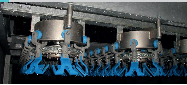
Kromeka air chilling lines can be designed for various live bird ranges and plant capacities, ranging from 1,000 - 13,500 bph. The use of high quality materials ensure trouble-free operation for many years. Refrigeration components such as evaporators and fans are all PLC controlled for easy and reliable operation.
